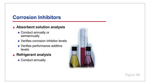
An absorption chiller requires a very deep vacuum to operate efficiently. The introduction of air and other noncondensables into the chiller will adversely affect the chiller's performance. In a lithium bromide absorption chiller, where the absorbent is a salt, corrosion is a potential problem that must be avoided. It may not be possible to completely prevent corrosion inside the chiller, although it can be reduced or controlled by the addition of a chemical called a **corrosion inhibitor**.
